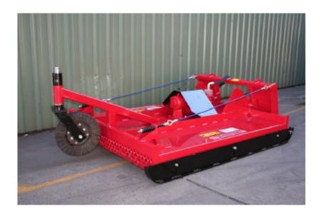
Hydrapower's 1500mm cut, 7601 Hydraulic Slasher Attachment is provided with quick attach frame to suit the carrier machine. The quick attach frame pivots on two bosses, allowing you to crowd the quick hitch forward when slashing to let the slasher deck follow the contours of the ground.
