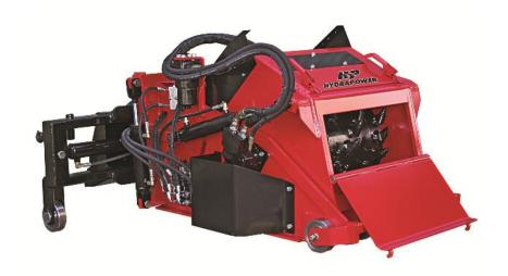
This state-of-the-art AC Profiler/Stabiliser is built with a John Deere/Cummins engine with 203hp. It has a working depth of up to 250mm and can run at 14/metres/minute at full depth, depending on road condition.
