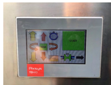
PLC on board for machine start-up. Touch screen and tilting of the turbine -20° +45°.
