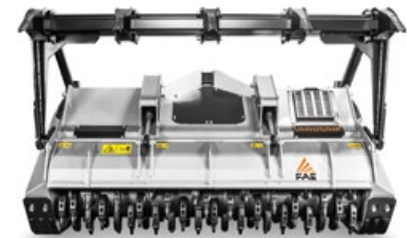
UMH/S - UMH/S/HP Forestry mulchers for PTO tractors with fixed tooth rotor.
